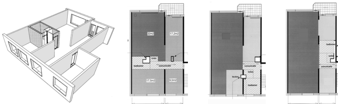
Figure 3: analyses of different scenarios for spatial organization of dwelling from 70's(left existing situation , last right the most wanted situation)
